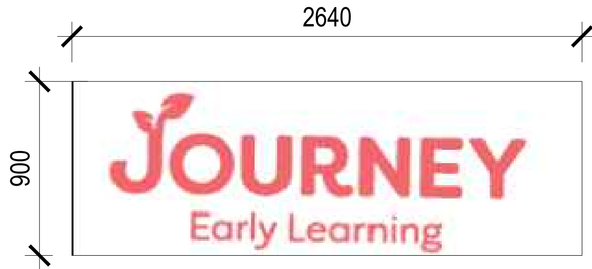
SIGN 1: 4mm WHITE ACM WITH 10mm ACRYLIC LETTERS PAINTED PINK (PMS184) ON ALL SIDES INCLUDING BACK. MECHANICALLY FIXED TO FACADE.
